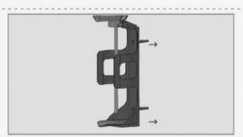
Snap the soap pipe from the dispenser body into the quick connection fitting of the pump.
